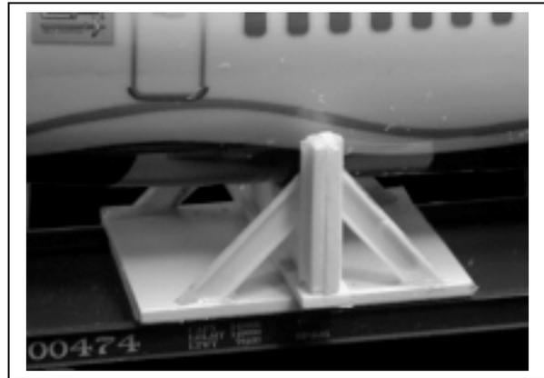
8 Position the Fuselage Support Assembly under the wing root as shown. After painting the fuselage you may attach the fuselage by gluing (
