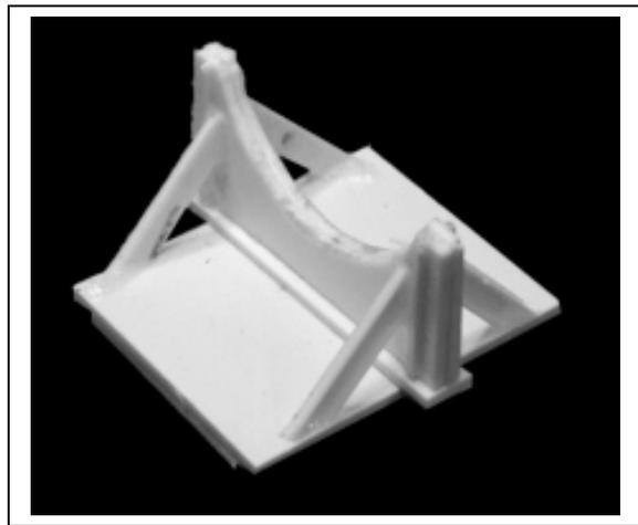
6 Add the Icicle Chopper to the leading end of the two car set. It will be necessary to remove cast-on grabs and other detail to get a flat surface to mount the Icicle Chopper. It will be necessary to file away the Icicle Chopper to get the correct width for the car being used.
