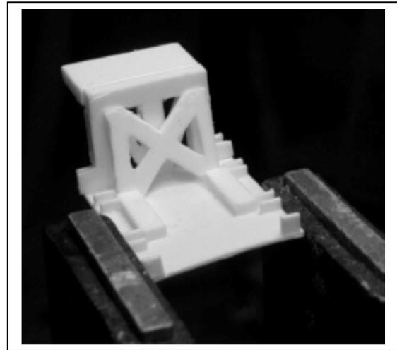
**3** Add the Longer Support (5) to the outside of the Vertical Mount. It will be necessary to file these parts for a good angle fit.
