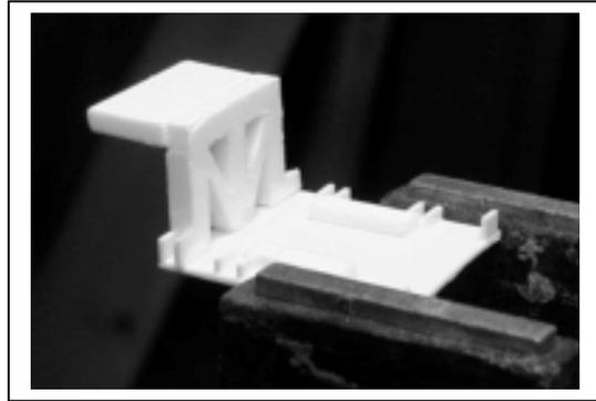
**2** Add the short brace as shown. It will be necessary to file it to fit. Note that it fits against the raised part of the Base Mount. Do Both Sides.
