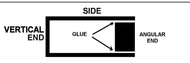
**4** Install the Bottom (6) by placing and gluing to the insides of the sides and ends. Now fit the Angular Tops (2,3) to the angled sides and ends. It will be necessary to finish filing for a good fit. Add the Top (9) to complete the structure. Use Squadron's Green putty to smooth all seams.
