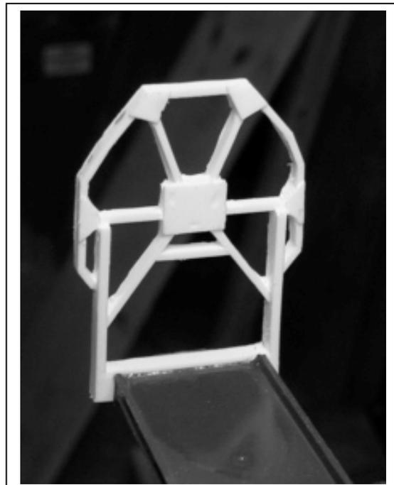
7 Position the Belly Support Assembly behind the front door of the fuselage approximately as shown.
