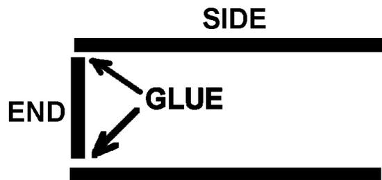
**3** Now glue the Angular End (7) to the angled portion of the sides. Refer to the photo at the top of the page. Install the Short End (8) at the bottom of the angled end.
